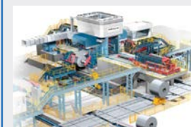
SMS Group cold rolling mill
